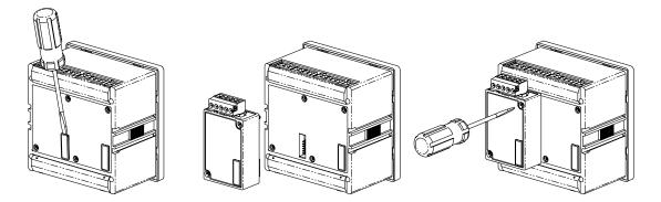
Connect the RI-F500/RI-F550 to the power supply, and then enter the module interface of the RI-F500/RI-F550 to check the information of slot X2. If the connection between the meter and the module is correct, the parameters of RI-A5ACDI will be shown.
