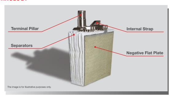
FIAMM FHT RANGE USE AGM (ABSORBED GLASS MAT) TECHNOLOGY. THE ELECTROLYTE IS ABSORBED IN FIBERGLASS SEPARATORS WITH 99% INTERNAL GAS RECOMBINATION EFFICIENCY. BLOCS ARE GRANTS NON-SPILLABLE AND MAINTENANCE FREE THEREFORE REQUIRES NO TOPPING UP OF ELECTROLYTE DURING ITS WHOLE LIFE. LOW SELF-DISCHARGE ALLOWS 6 MONTHS SHELF LIFE.
