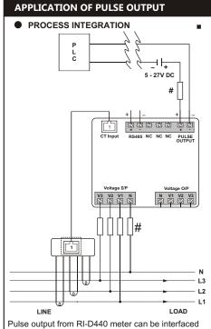
Pulse output from RI-D440 meter can be interfaced into a process through a PLC for on line control of energy content in the process.
