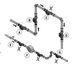
In order to avoid cavitation, the back pressure at the flow sensor (the pressure at the flow sensor outlet) must be minimum 1.5 bar at  $q_p$  (nominal flow) and minimum 2.5 bar at  $q_s$  (maximum flow). This applies to temperatures up to approx. 80 °C. The flow sensor must not be exposed to pressure lower than the ambient pressure (vacuum).
